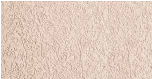
Rustic texture produced with Ceresit CT 35 mineral plaster, grain size 2.5 mm, obtained by circular floating with a plastic float
