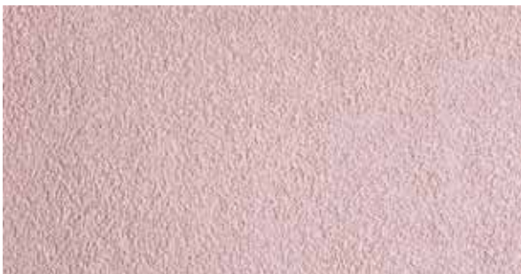
Stone texture produced with Ceresit CT 60 acrylic plaster, grain size 1.5 mm, obtained by floating with a plastic float
