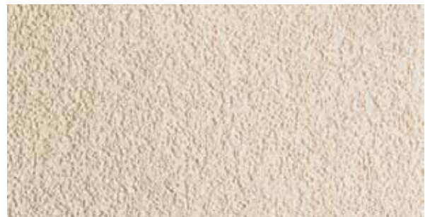
Stone texture produced with Ceresit CT 137 mineral plaster, grain size 2.5 mm, obtained by floating with a plastic float
