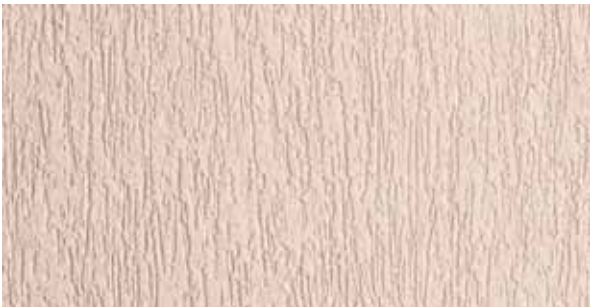
Rustic texture produced with Ceresit CT 35 mineral plaster, grain size 2.5 mm, obtained by floating with a plastic float in one direction
