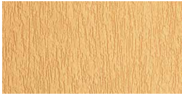
Rustic texture produced with Ceresit CT 64 acrylic plaster, grain size 2.0 mm, obtained by floating with a plastic float in one direction
