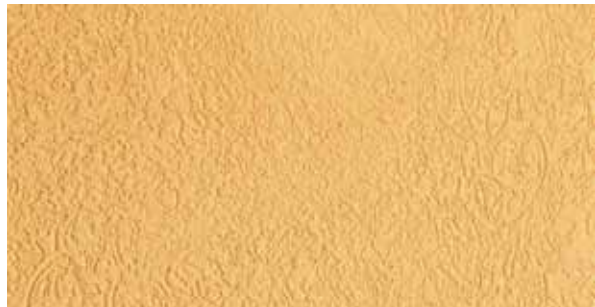
Rustic texture produced with Ceresit CT 64 acrylic plaster, grain size 2.0 mm, obtained by circular floating with a plastic float
