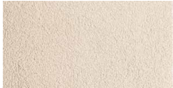
Stone texture produced with Ceresit CT 137 mineral plaster, grain size 1.5 mm, obtained by floating with a plastic float
