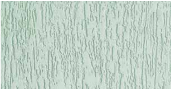
Rustic texture produced with Ceresit CT 63 acrylic plaster, grain size 3.0 mm, obtained by floating with a plastic float in one direction
